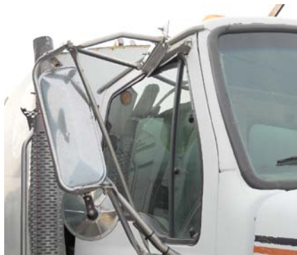
Damage to ID truck due to encroaching branches.
